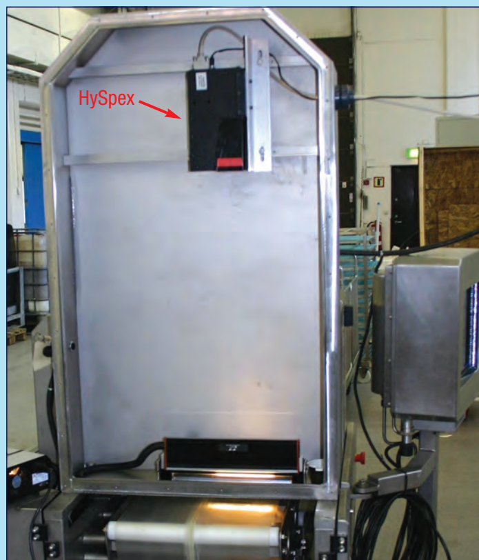
Figure 13. A HySpex camera mounted above a conveyer belt in an industrial application.
