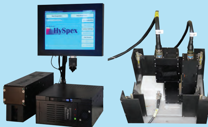
Figure 5. To the left; the ultra-compact DAU for airborne applications (10.5 x 20.5 x 25 cm), HySpex VNIR-1600 and the trans-reflective touch-screen. The total power consumption of this system is less than 75 W. To the right; HySpex VNIR-1600 and HySpex SWIR-320m-e mounted in a vibration damped platform, together with an IMU/GPS unit.
