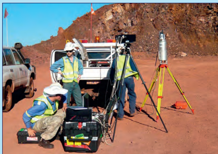
Figure 10. HySpex camera and LIDAR set up for mine face scanning.
